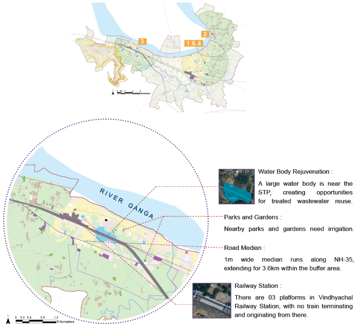
Figure 37: Identified Bulk Users in Accessible Radius of STP 3 - Vindhyachal
